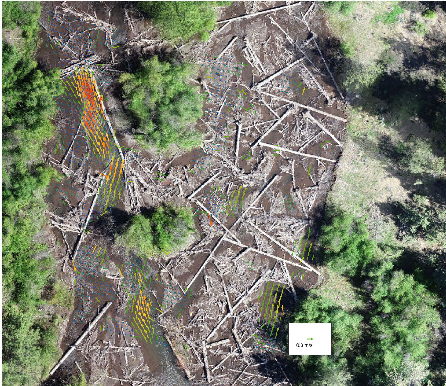
Figure 4. PIV-derived flow velocity vectors (m/s) and number of vectors per 0.05 m/s bin along 70 m valley length of the Whychus Canyon Phase 2a restoration reach showed high heterogeneity in velocities and a high proportion of velocity vectors with velocities less than 0.3 m/s, the upper limit of optimal velocity for rearing salmon and trout.
