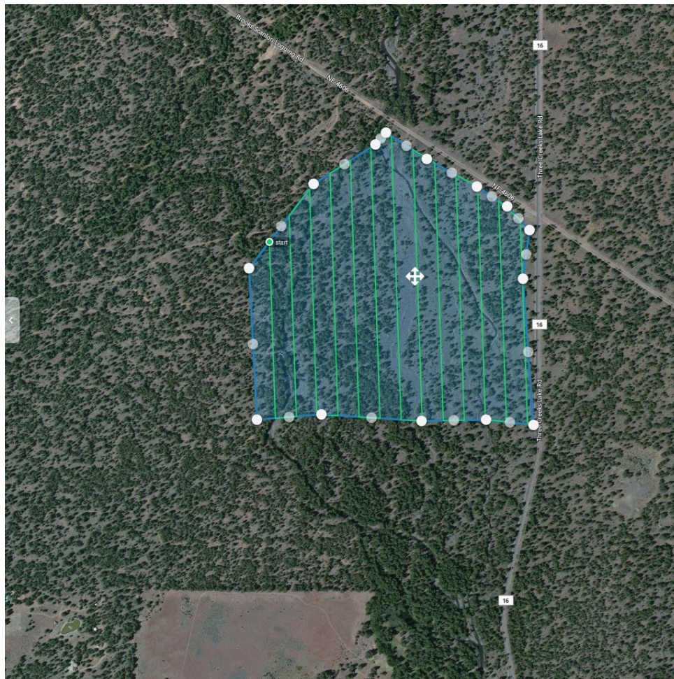
Figure 1a. Example of the arrangement of flight lines for a mission South of Sisters, OR. Green lines show the planned flight direction of the UAV.
